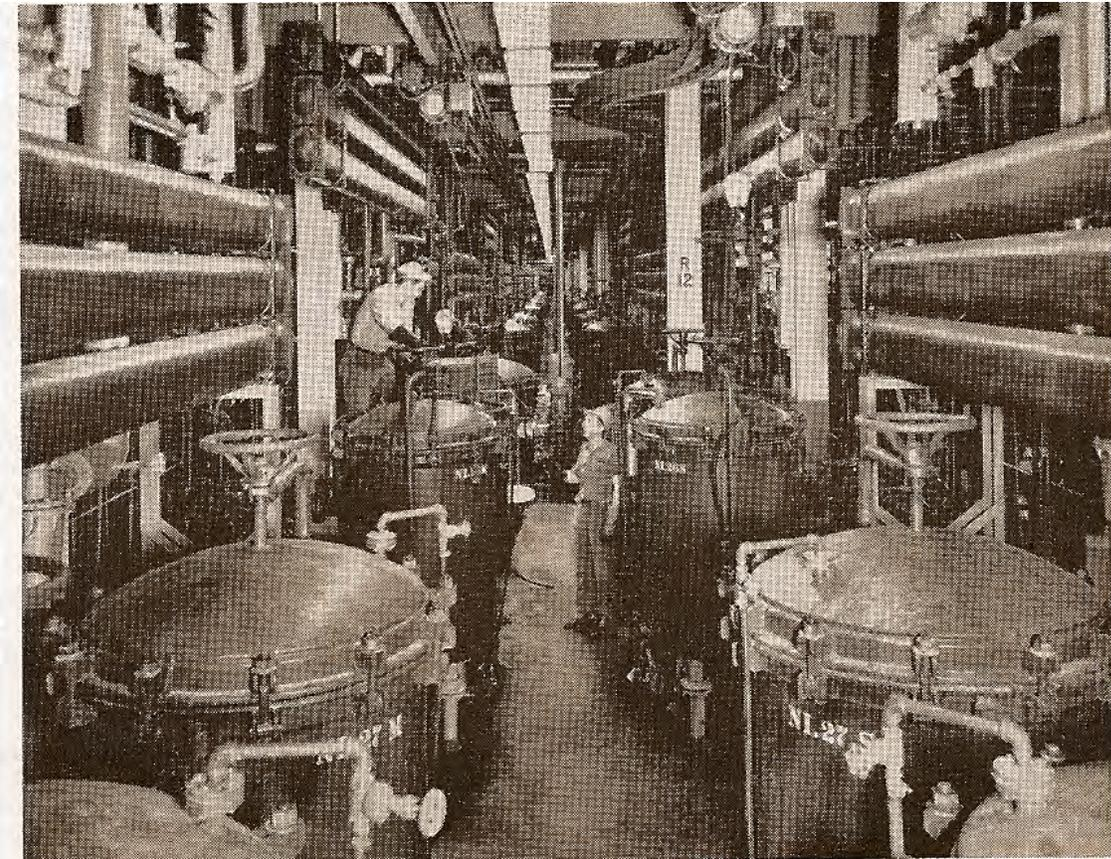
This Article deals with batch pressure filters (Above) that utilize filter elements that are enclosed in a liquid- and vapor-tight tank. This enclosed type of filter offers obvious advantages over the old plate-and-frame press type of batch pressure filter.
