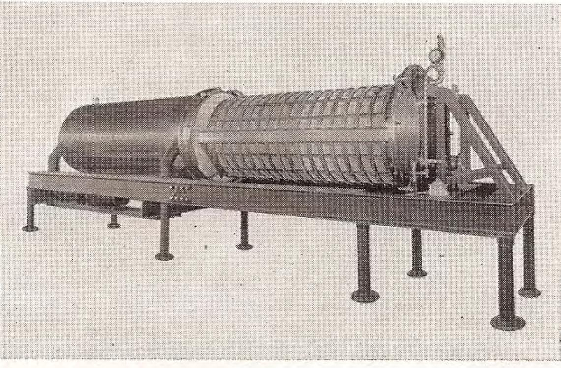
Vertical Element Filters, such as shown in photographs (Immediately Above) can be constructed of a variety of materials to meet particular process requirements. They can also be constructed with a lined tank for added corrosion resistance, if necessary. Sizes of these filters range from 100 to 2,000 sq. ft. of filtration area in one unit.
